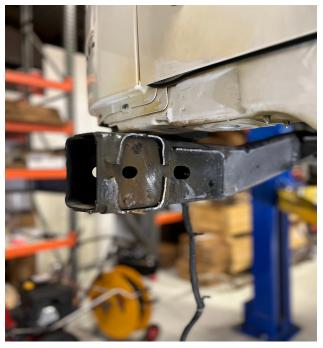
5.)Using a flap wheel remove any remaining portion of the cross member and body mount until the frame is smooth.
